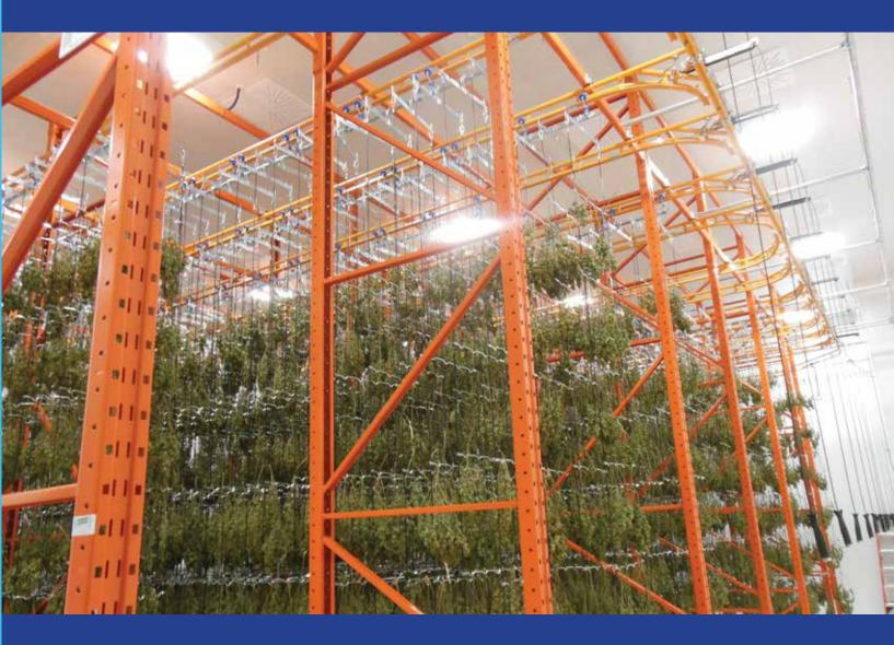
Engineering Solutions For All Your Hang-Ups www.srsconveyors.com sales@srsconveyors.com SRS Conveyors is pleased to introduce our innovative plant drying rail system. **The Cannabis Trolley Transport System** provides an effective material handling solution for storing and transporting cannabis plants during the harvesting, drying, and trimming processes of cannabis production.
