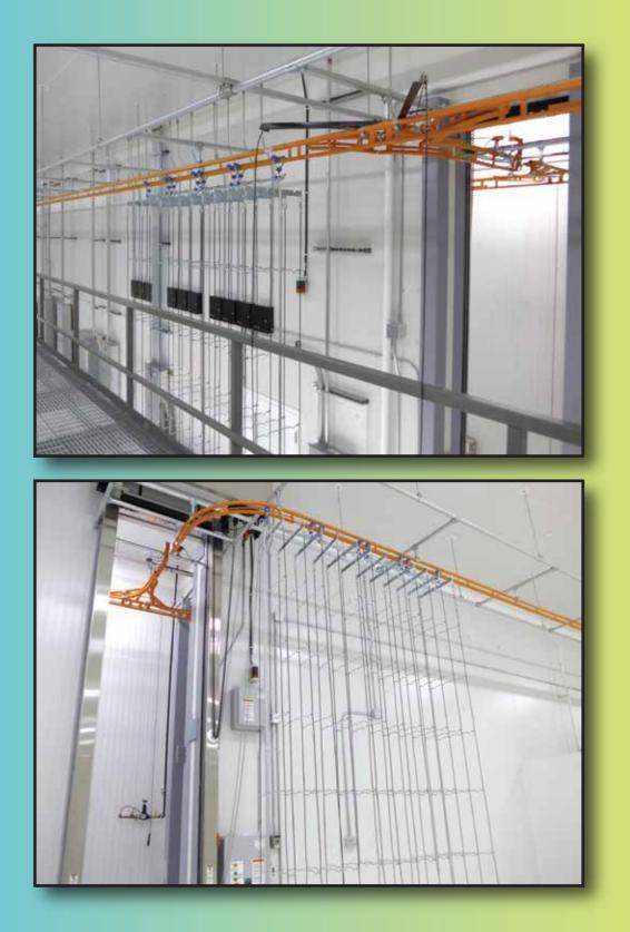
The system creates an efficient flow of material while maximizing the use of available vertical space in your facility. Plants are hung on multi-tiered rolling trolleys, which can link together to form a train. This enables you to carry and transport thousands of cannabis plants at once. The trolleys can be left directly inside humidity controlled drying rooms, eliminating the lengthy step of hanging and collecting plants between each production phase.
